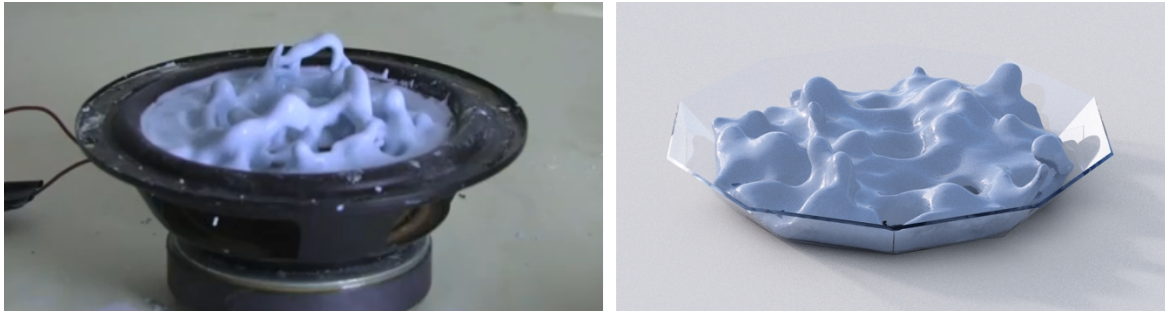
Figure 5: Vibration experiment with a shear thickening fluid. The images show a comparison between the real experiment results [41] (left image) and our results obtained in simulation (right).
