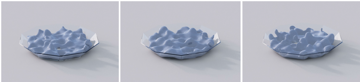
Figure 6: The snapshots from the vibration experiment with our shear thickening fluid model show the expected finger-like formations with various shapes. These formations do not appear if the history terms are removed.
