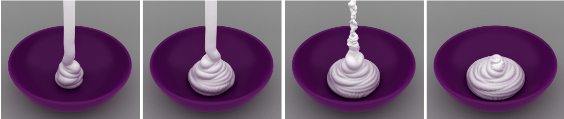
Figure 12: In simulations that do not include high energy interactions the result resembles a standard viscoelastic fluid.
