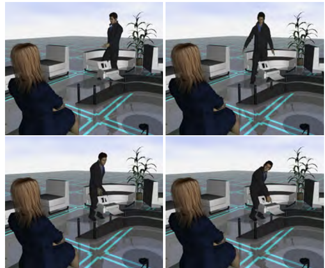
Figure 32: The PLACE planner synthesizes whole-body demonstrations for arbitrarily located targets and observers, also taking into account obstacles and visual occluders.
