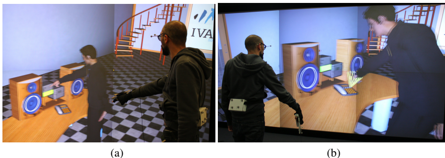
Fig. 1. (a) In this scenario, during the modeling phase, the user demonstrates several examples of pointing motions in order to demonstrate operations with a stereo system and a telephone. (b) During the training phase, the user requests the virtual human to precisely perform the same pointing motions for arbitrary targets, here specified by the apex of the yellow cone which is controlled via a WiiMote controller. The training phase is used here to test if the example motions are sufficiently covering the volume of interest in the scenario. The user can interactively switch between the two phases until all required motions are correctly defined. Note that the simulated images in this figure appear fuzzy since they are being projected for stereo visualization.
