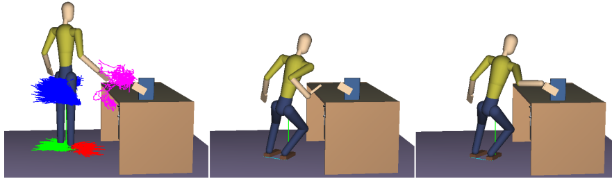
Fig. 10 In this example, a large k_1 value was used allowing many expansions in the bidirectional searches and leading to a relatively complex reaching motion being found. By using smaller values for k_1 , more mobility skills would be recruited favoring reaching solutions needing fewer bidirectional expansions to reach the goal. The colored trajectories illustrate the locations traversed by the joints controlled by each skill instantiated in T .
